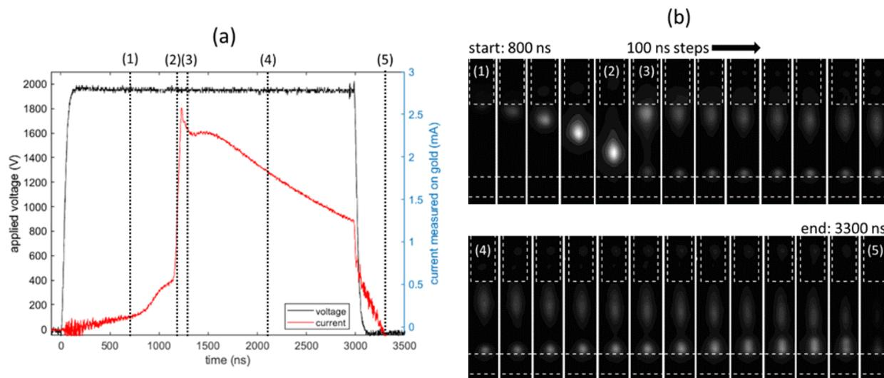
Supplementary Figure 2. Data showing the time-dependent behavior of the plasma jet interacting with a gold substrate. (a) Shows the pulsed-DC voltage applied to the plasma jet along with the current measured on the substrate and (b) shows the high speed images of the jet interacting with the substrate. The vertical lines in (a) indicate corresponding images shown in (b).
