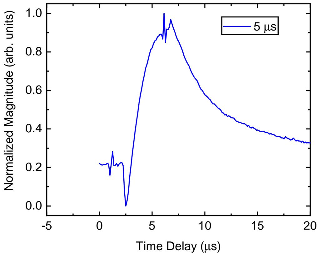
Supplementary Figure 3. Thermoreflectance measurement data at a laser probe wavelength of 405 nm. Due to the positive thermoreflectance coefficient of Au at this wavelength, these data show a decrease in reflectance during cooling and increased reflectance as the sample temperature increases.
