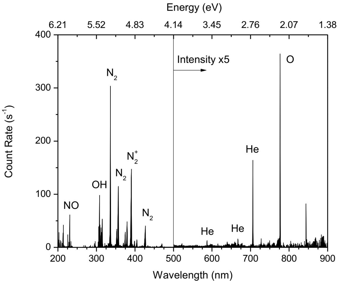
Supplementary Figure 5. Emission spectrum of a plasma jet produced in helium interacting with a gold substrate. The spectrum is acquired near the jet exit through a line of sight perpendicular to the axis of the jet. The intensity of the spectrum for wavelengths above 500 nm has been multiplied by 5.
