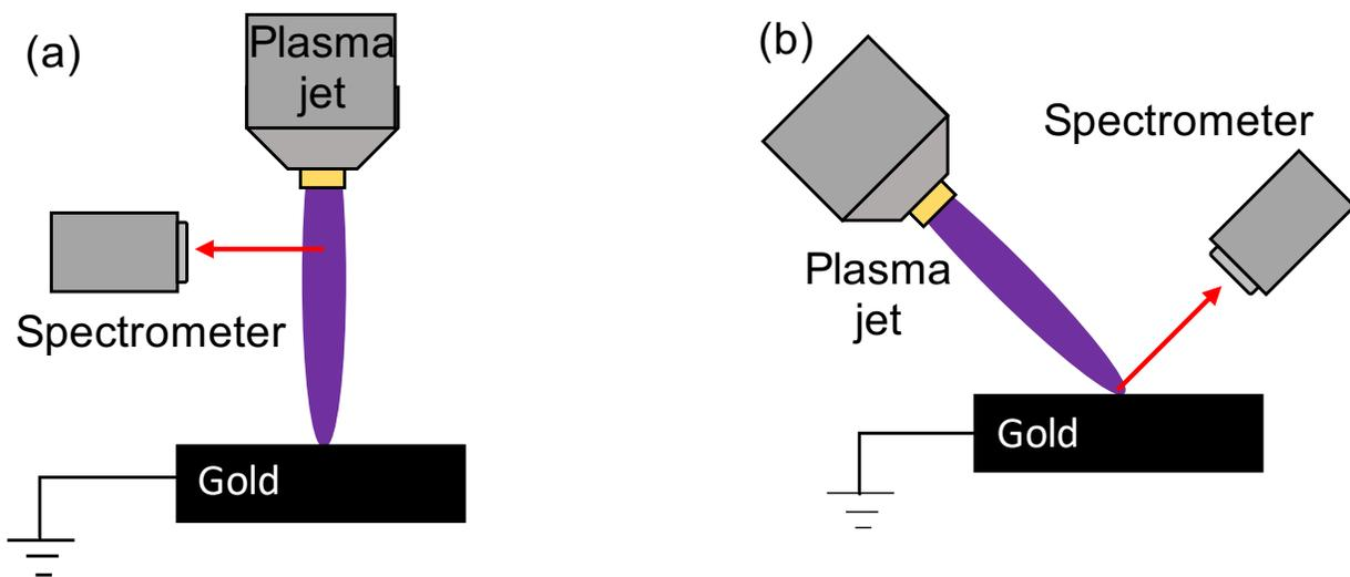
Supplementary Figure 4. Experimental configurations for measuring optical emission spectra of the plasma jet in this work. (a) Shows a typical geometry where the emission spectra is acquired through a line of sight normal to the axis of the jet. This geometry was used to acquire the spectrum in Fig. S2(b). (b) Geometry used to acquire time-dependent emission spectra as seen by the surface and shown in Fig. 3(a) of the manuscript.
