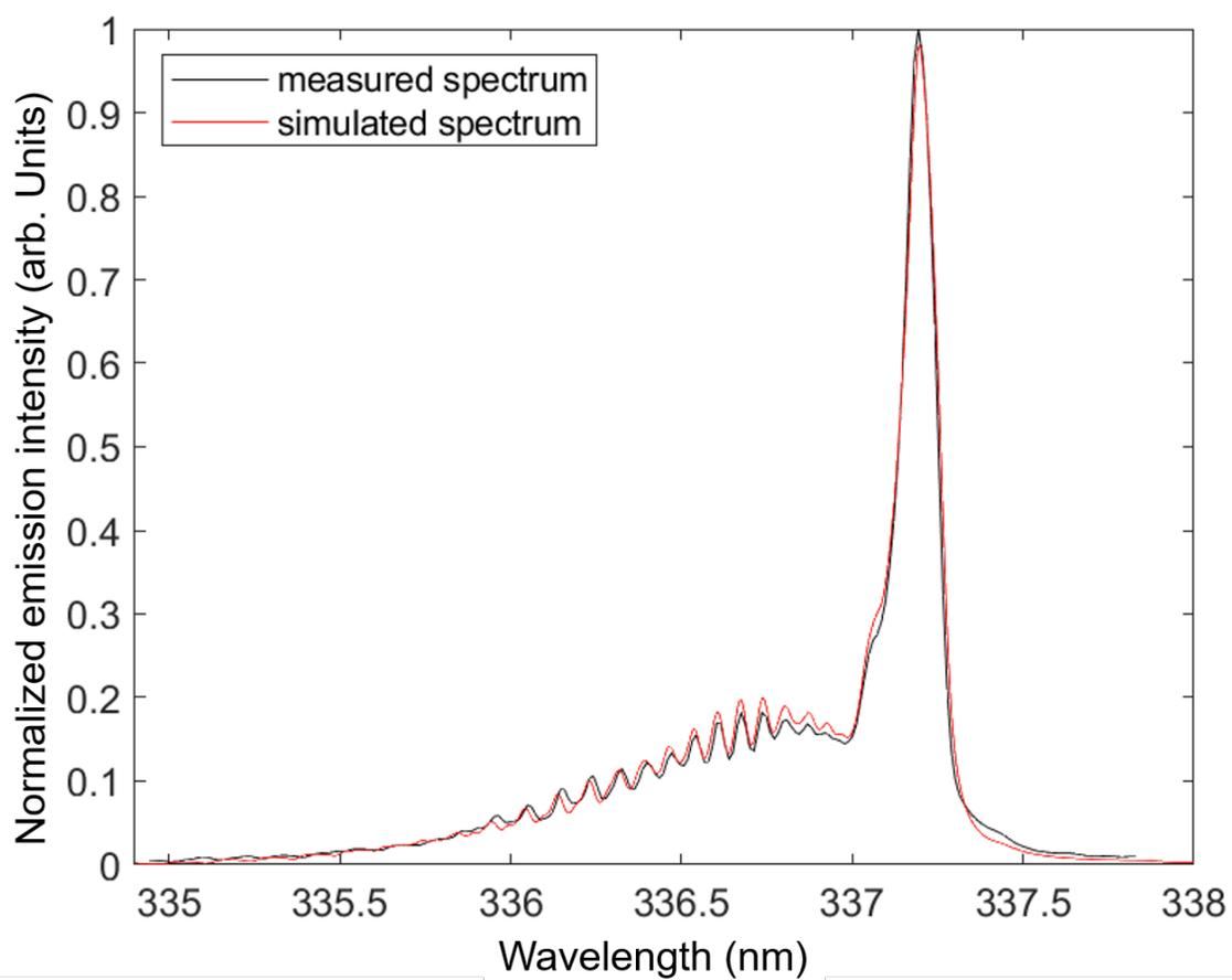
Supplementary Figure 6. N<sub>2</sub> emission spectrum. The measured and simulated emission spectra of the 337 nm line of the second positive system in N<sub>2</sub> [N<sub>2</sub>(C<sup>3</sup>Π<sub>u</sub> → N<sub>2</sub>(B<sup>3</sup>Π<sub>g</sub>)].
