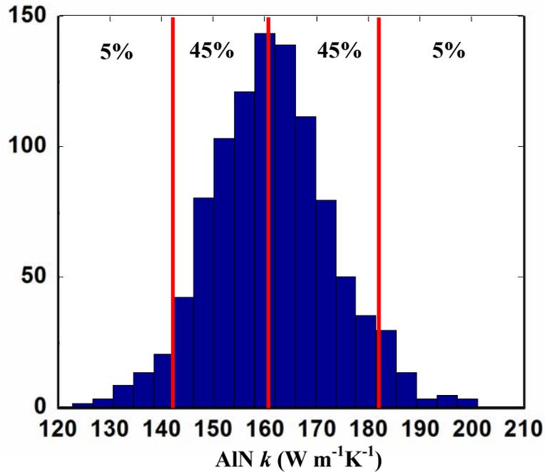
Figure S4. Monte Carlo error bar calculation with 1000 times of data fitting. The data is for Samp\_4 at 380 K. 90% percentile confidence interval (AlN thermal conductivity =161.1-18.3/+20.7 W/m-K).
