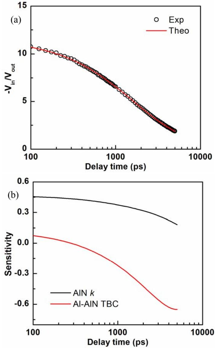
Figure S3. (a) TDTR data fitting of Samp\_4 at room temperature with 3.6 MHz. (b) TDTR sensitivity of AlN thermal conductivity (AlN  $k$ ) and Al-AlN thermal boundary conductance (Al-AlN TBC). High sensitivity here results in accurate measurements.
