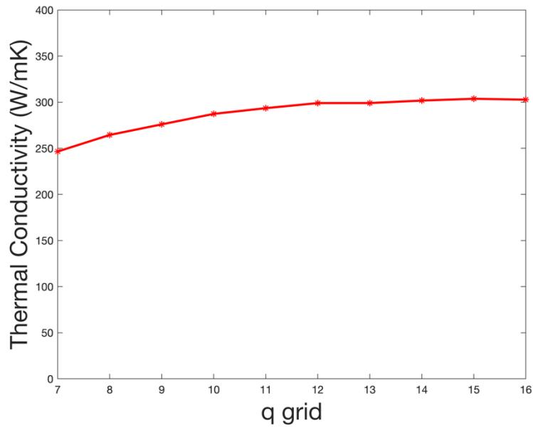
Figure S5. Thermal conductivity of AlN with  $q$  grid used in the DFT calculation.
