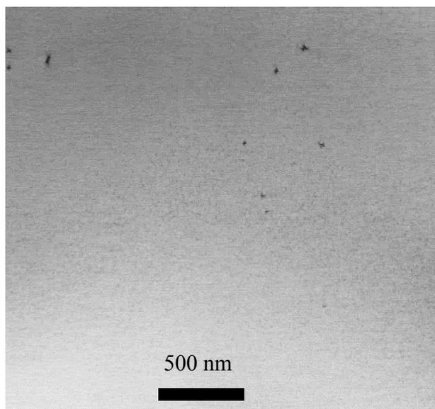
Figure S1. Near-surface plan-view (11 $\bar{2}$ 0) two-beam condition STEM image of Samp\_1. The black dots in this image are dislocations. The dislocation density is  $\sim 1.6 \times 10^8/\text{cm}^2$ .
