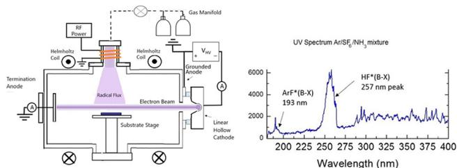
**FIG. 1.** (Left) Schematic of the LAPPS configuration with an auxiliary inductively coupled plasma radical source. (Right) UV spectrum of  $\text{Ar/SF}_6/\text{NH}_3$  plasma showing the presence of excited HF molecules.
