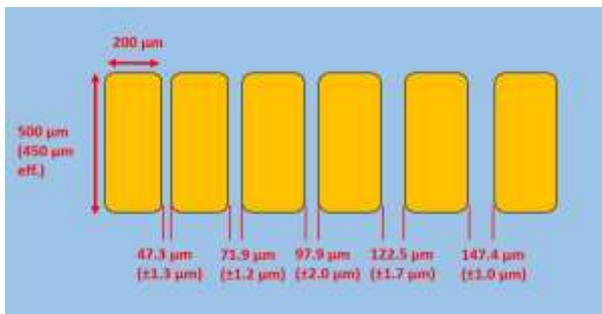
**Figure S5.** Top view of TLM structure
