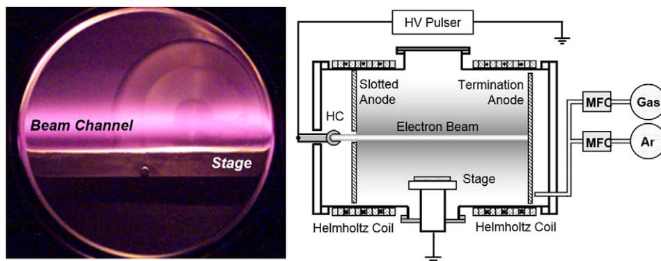
**Fig. 1.** The large area plasma processing system (LAPPS), which employs an electron beam generated plasma. (Left) An image of the plasma, and (Right) a schematic diagram of the processing reactor used in this work.
