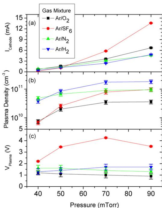
**Fig. 3.** Characteristics of electron beam generated plasmas produced in a variety of gas mixtures as a function of operating pressure. The indicated reactive gas is 5% by flow. Shown are (a) the cathode current along with corresponding (b) charged particle density and (c) plasma potential. The increase in plasma density and minimal change in plasma potential with pressure suggest an increase in ion and reactive neutral flux at the surface but no change in ion energy as pressure increases.
