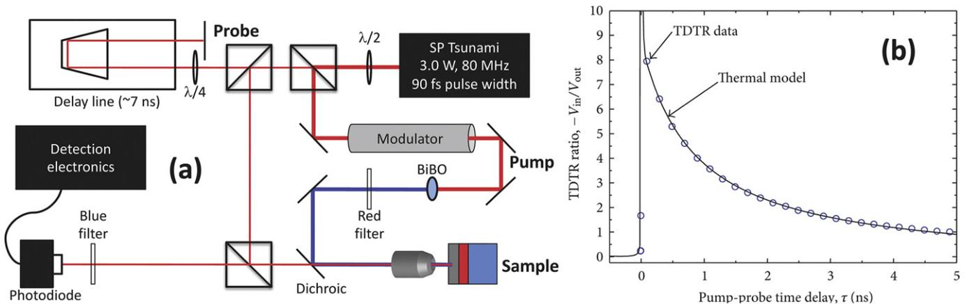
Fig. 2. (a) Major components in the TDTR experiments as described in the text along with (b) example TDTR data.
