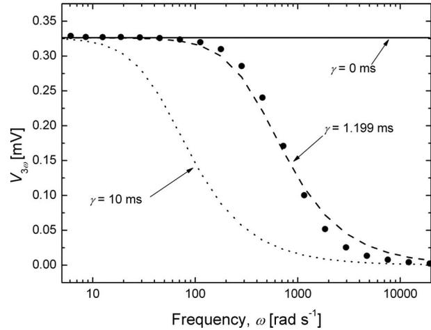
**Fig. 3 Sensitivity of Eq. (1) to the thermal time constant  $\gamma$ . A best fit thermal conductivity  $k$  is 66  $\text{W m}^{-1} \text{K}^{-1}$ . The thermal conductivity of the test structures is easily determined by identifying the region of frequency independent  $V_{3\omega}$  and fitting Eq. (2) to the data.**
