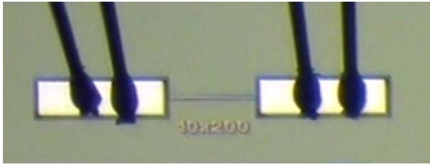
**Fig. 1** Optical microscope image of a 10  $\mu\text{m}$  wide  $\times$  200  $\mu\text{m}$  long test structure fabricated using the SUMMiT V<sup>TM</sup> process. The bond pads are 100  $\mu\text{m}$  wide and 300  $\mu\text{m}$  long. Two wires bonded to bond pad are visible in the image. The connections to the package are outside of the image.
