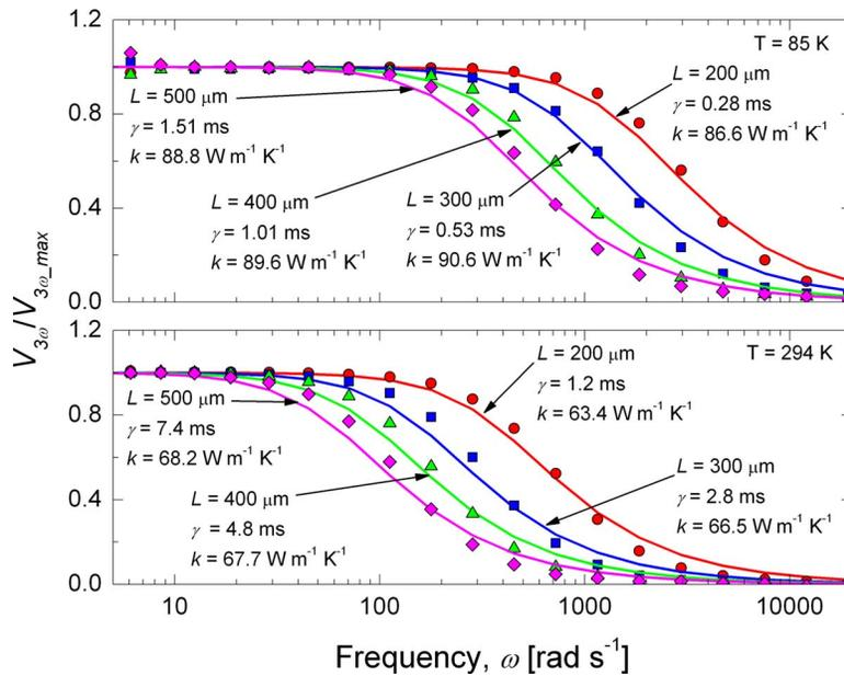
**Fig. 4**  $3\omega$  voltage on the different length bridge structures with the Eq. (1) fit to the data with best fit  $k$  and  $\gamma$ . The data and best fit are normalized for clarity. The frequency independent region of the  $3\omega$  voltage responses increases with a decrease in temperature.
