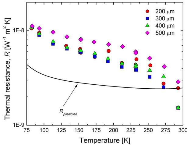
**Fig. 8 Additional thermal resistances determined from the two data sets in Fig. 7 and Eq. (7) compared with the predicted thermal resistance  $R_{\text{predicted}}$  of the 700 nm Al bond pad the Al/Si interface**
