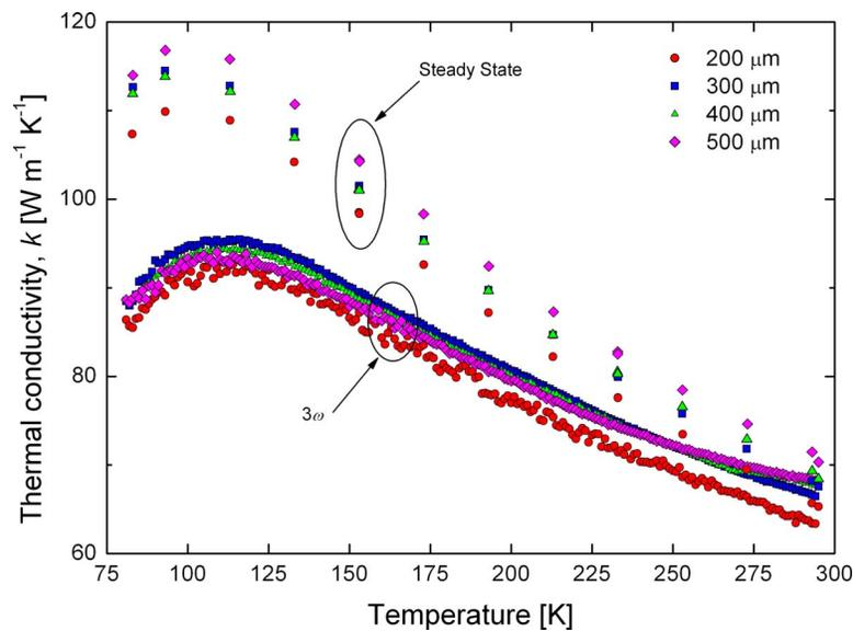
**Fig. 7** Temperature dependent thermal conductivity data on the polysilicon bridge test structures. The  $3\omega$  and steady state measurements are both presented for comparison. The differences between the two sets of data determined from the different measurement techniques can be explained by the effects of bond pad heating and thermal boundary resistance between the Al wire bonded film and the bond pad.
