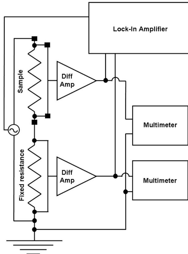
**Fig. 2** Schematic representing circuit and data acquisition equipment in the  $3\omega$  measurements. The sample is the polysilicon microbridge structure, and the fixed resistance varied depending on the sample. The value of the fixed resistance was chosen to be slightly higher than the maximum resistance across the sample [14]. During testing, this value was set to be slightly higher than the room temperature resistance of the sample.
