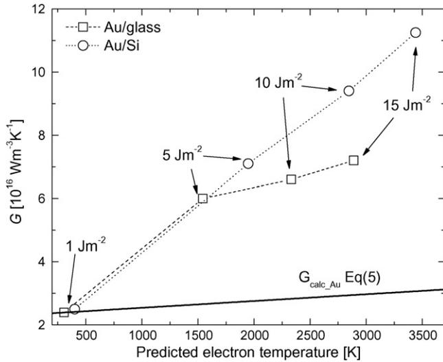
Fig. 3. Best fit  $G$  for 20 nm Au on Si and glass at several different laser fluences. The large divergence of the measured  $G$  using the TTM from that predicted  $G$  using Eq. (5) could be a result of a nonequilibrium between the electrons and substrate causing another channel for energy transfer away from the electron system.
