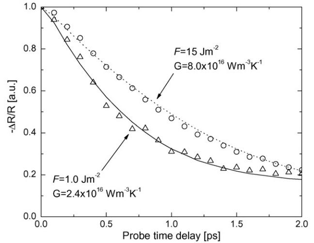
Fig. 2. TTM fit to the first 2.0 ps of the data in Fig. 1. The best fit resulted in drastically different  $G$ 's for the two laser fluences.
