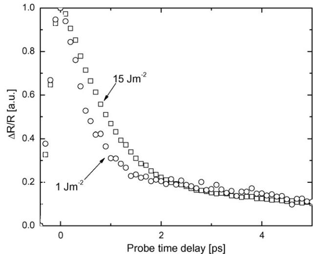
Fig. 1. Phase corrected TTR data on a 20 nm Au/glass sample taken at two laser fluences. The data is normalized at the peak reflectance to show the difference in cooling profiles of the electron systems during the first few picoseconds after laser heating. The initial time ( $t_0$ ) is defined at time of peak reflectance.
