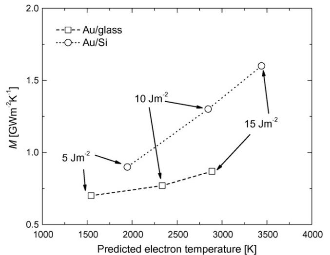
Fig. 4. Rate of energy loss from the electron system beyond e–p coupling,  $M$ , deduced from the 3TM applied to TTR data assuming a  $G$  temperature dependence in accordance with Eq. (5). The electron system energy loss is always greater on the semiconducting Si substrate than on the insulating glass substrate.
