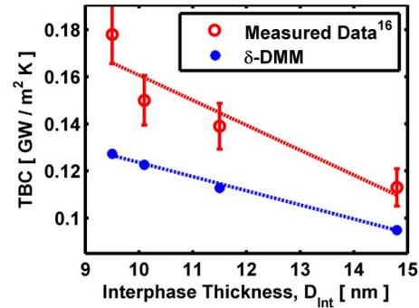
FIG. 3. (Color online) Comparison of thermal boundary conductance measurements made on a series of Cr/Si interfaces [Hopkins *et al.* (Ref. 16)] with predictions obtained from the  $\delta$ -DMM. Predictions using the  $\delta$ -DMM correlate far better than those obtained using the standard DMM (DMM of Cr/Si=0.86 GW/m<sup>2</sup> K), while capturing the dependence of interfacial conductance on the thickness of disorder.
