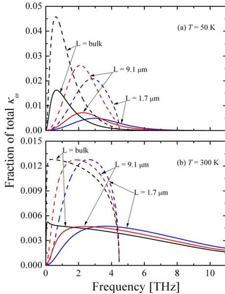
FIG. 2. (Color online) Fraction of the total spectral thermal conductivity at (a) 50 and (b) 300 K for  $L = \infty$  (no void boundaries), 9.1, and 1.7  $\mu\text{m}$ , where  $L$  is the distance between void boundaries. The longitudinal components are shown by the solid lines and the transverse components by the dashed lines.
