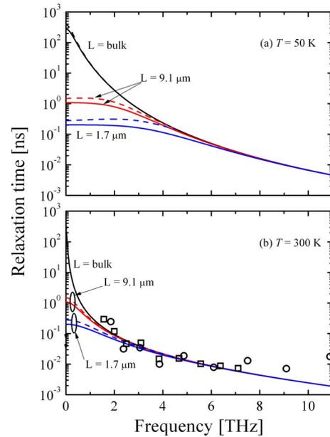
FIG. 3. (Color online) Relaxation time of the longitudinal (solid lines) and transverse (dashed lines) as a function of frequency for (a)  $T = 50$  K and (b)  $T = 300$  K. For comparison, relaxation times calculated with MD simulations for bulk Si at 300 K are shown (Ref. 21). The circles represent the longitudinal modes and the squares the transverse modes.
