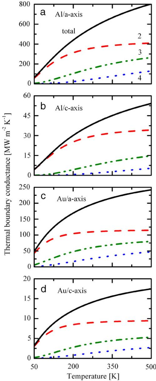
**Fig. 1.** Temperature-dependent  $h_{BD}$  at Al–graphite and Au–graphite interfaces for both orientations of graphite, as well as the individual contributions from two-, three-, and four-phonon processes. Higher-order inelastic phonon processes become more significant to the overall value of  $h_{BD}$  with increased temperature, as well as increased acoustic mismatch (the Au–graphite mismatch is greater than that of Al–graphite).
