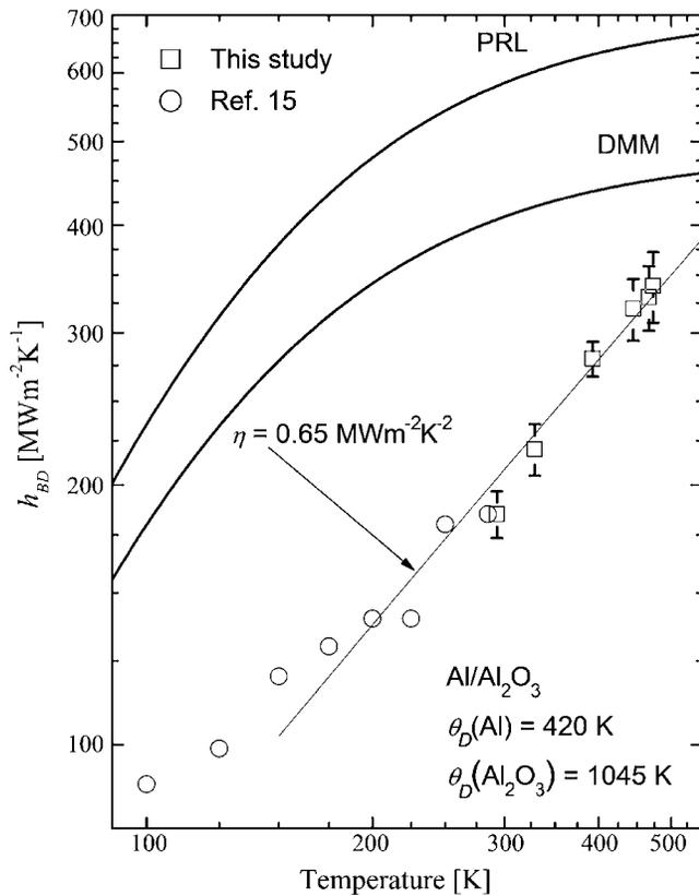
**Fig. 5** Thermal boundary conductance data across the Al/Al<sub>2</sub>O<sub>3</sub> interface over a range of temperatures. This figure also includes data taken by Stoner and Maris (1993) at low temperatures [15]. The linear trend continues at temperatures higher than the Debye temperature of Al, indicating that inelastic phonon processes could be contributing to  $h_{BD}$  at these elevated temperatures.
