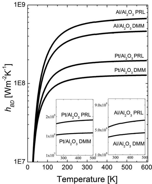
**Fig. 1 Thermal boundary conductance calculations of the Al/Al<sub>2</sub>O<sub>3</sub> and Pt/Al<sub>2</sub>O<sub>3</sub> interfaces using DMM and PRL. The models level off at higher temperatures due to the assumption of elastic scattering used in the calculations. The inset graphs show the DMM and PRL for the materials systems over only the temperature range used in this work.**
