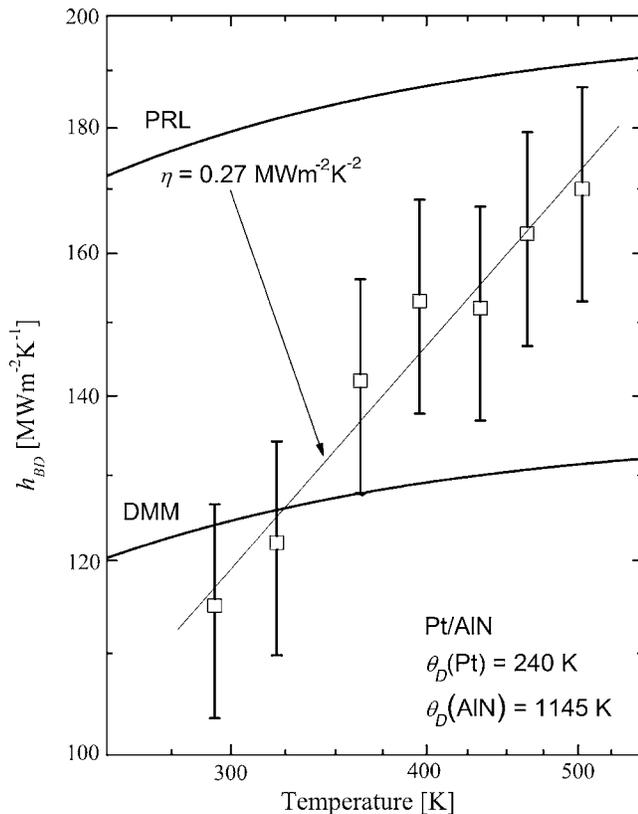
**Fig. 7 Thermal boundary conductance data across the Pt/AlN interface over a range of temperatures. A similar linear increase of  $h_{BD}$  to the data in Fig. 7 is observed, presenting further evidence toward nonelastic phonon transport channels.**
