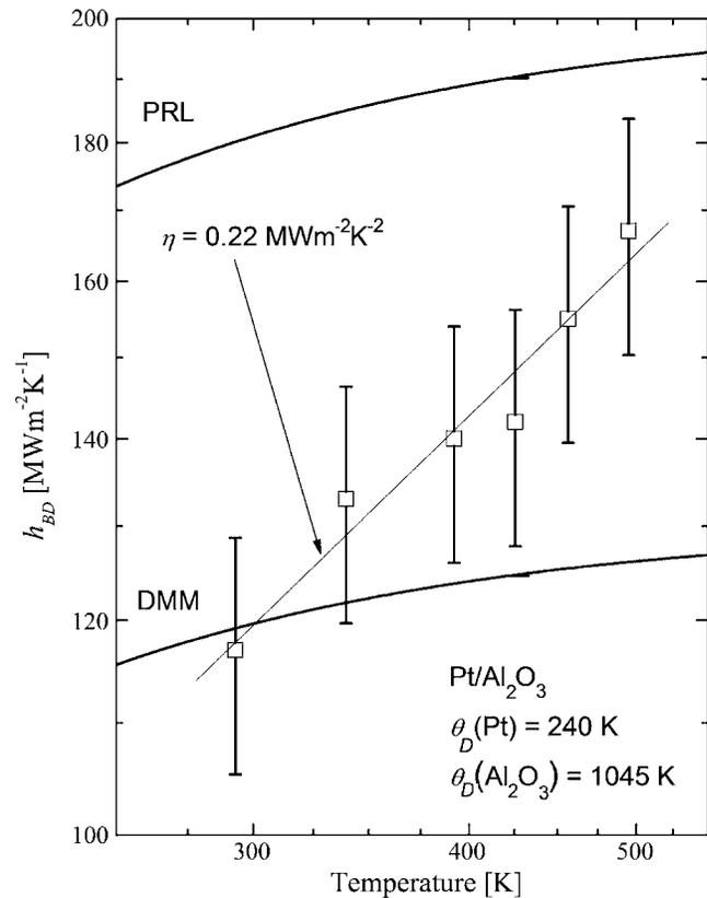
**Fig. 6** Thermal boundary conductance data across the Pt/Al<sub>2</sub>O<sub>3</sub> interface over a range of temperatures. These temperatures are above the Debye temperature of Pt. According to theory,  $h_{BD}$  should not change at temperatures above the Debye temperature of one of the materials assuming only elastic scattering. However, the continued linear increase in measured  $h_{BD}$  indicates a contribution from inelastic processes.
