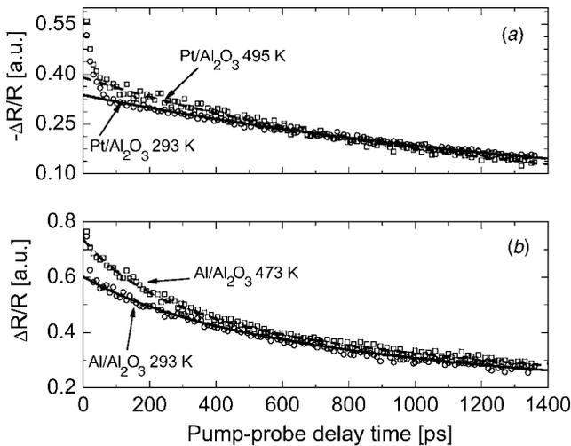
**Fig. 3** Thermal model (Eqs. (8)–(14)) fit to TTR data taken on (a) Pt/ $Al_2O_3$  at 293 K and 495 K and (b) Al/ $Al_2O_3$  at 293 K and 473 K. The thermal model is scaled to the TTR data at 200 ps for reasons that will be discussed later in this paper. The TTR data were phase fixed [29] and normalized at the peak reflectance to make clear the differences in the exponential cooling profiles at the different temperatures.
