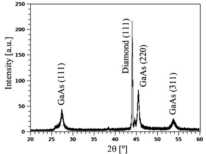
FIG. 3. Omega-2 theta XRD scan of a 5- $\mu\text{m}$ -thick GaAs growth on CVD diamond. The diamond (111) plane and the GaAs (111), (220), and (311) planes are clearly developed.
