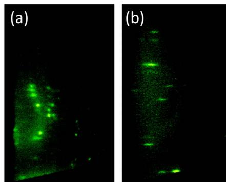
FIG. 1. (Color online) Reflective high-energy electron diffraction pattern of (a) CVD-diamond substrate and (b) GaAs on CVD diamond. The RHEED pattern shows a highly polycrystalline CVD-diamond substrate and the GaAs layer also shows a similar polycrystalline signature with more streaks indicating reduced roughness.
