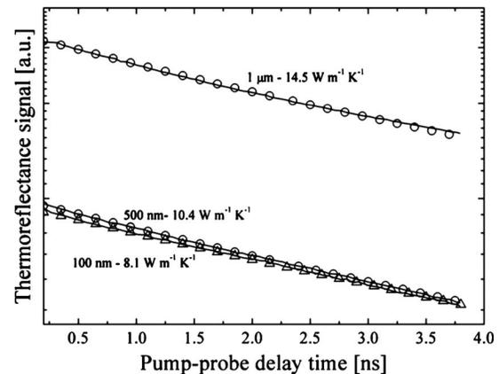
FIG. 4. Thermal conductivities of 1  $\mu\text{m}$ , 500 nm, and 100 nm poly-GaAs films on CVD diamond as measured using pump-probe time domain thermoreflectance.
