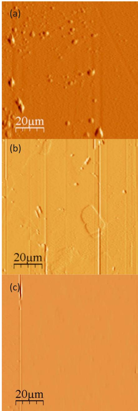
FIG. 2. (Color online) AFM surface scans of (a) CVD diamond, (b) poly-GaAs on CVD diamond, and (c) polished poly-GaAs on CVD diamond. The surface roughness reduces significantly in the three cases: from  $>50$  nm rms for the diamond, to 10–15 nm for the poly-GaAs on the diamond, to finally 1–5 nm rms for the polished poly-GaAs on diamond.
