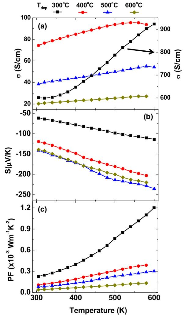
**Fig. 2.** (Color online) (a) Electrical conductivity vs temperature ( $\sigma$ - $T$ ) characteristics, (b) Seebeck coefficient vs temperature ( $S$ - $T$ ) characteristics, (c) power factor vs temperature (PF- $T$ ) characteristics of AZO thin films deposited at different temperature ( $T_{\text{dep}} = 300, 400, 500,$  and  $600^\circ\text{C}$ ).
