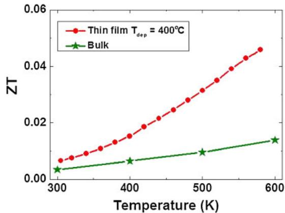
**Fig. 5.** (Color online) Dimensionless figure of merit at elevated temperatures using thermal conductivity at 300 K for AZO thin film deposited at 400 °C compared with our previously reported bulk material<sup>16</sup> of same composition.
