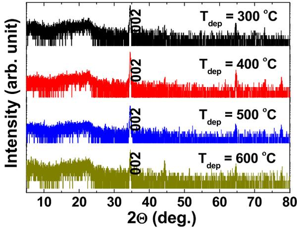
**Fig. 1.** (Color online) XRD patterns of AZO films deposited at different temperatures ( $T_{\text{dep}} = 300, 400, 500,$  and  $600^\circ\text{C}$ ).
