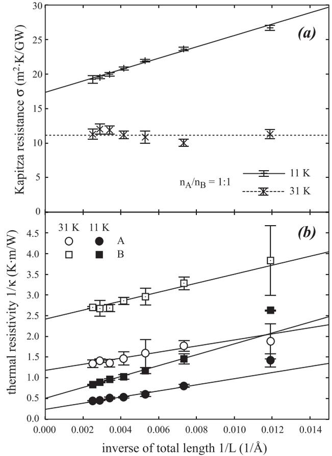
FIG. 2. Kapiza resistance (a) and component resistivities (b) as a function of inverse of system length for the LJ bicrystal, where only the atomic mass differs. The mass of the B component of the bicrystal is 3 times the mass of A, which is nominally the mass of Ar.
