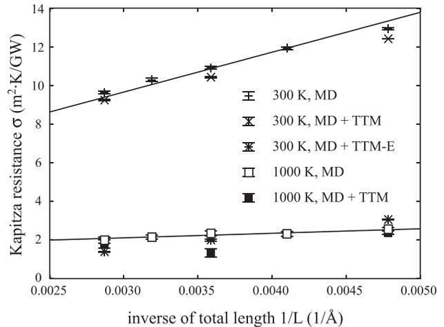
FIG. 3. Al:GaN resistances as a function of total length at 300 K and 1000 K for different two temperature coupling (none: “MD,” e-ph coupling in Al only: “MD+TTM,” e-ph coupling in Al + 1 unit cell overlap with GaN: “MD+TTM-E”).
