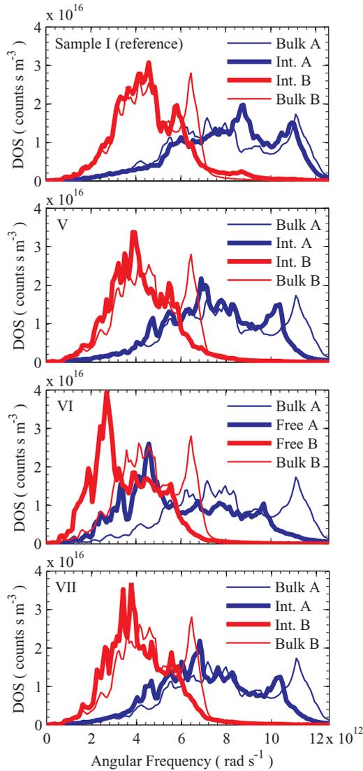
FIG. 2. (Color online) Phonon density of states curves at 12 K calculated via Eq. (1) within the monolayers adjacent to the interface (heavy lines) compared to bulk (light lines). A reduction in either  $r_{c,AB}$  or  $\epsilon_{AB}$  causes a softening of modes on both sides of the interface.
