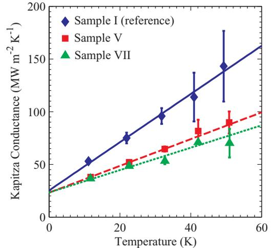
FIG. 1. (Color online) Temperature-dependent  $h_K$  data from NEMD simulations for samples I, V, and VII. Each data point is the average over three to five independent simulations and error bars represent the standard deviation, i.e., repeatability. Solid and dashed lines are linear fits of the data. While the slopes of these linear fits exhibit strong dependence on cross-species interaction parameters, the  $y$  intercepts do not.
