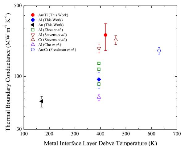
FIG. 3. Comparison of room temperature thermal boundary conductances across various metal-GaN interfaces as a function of interface metal Debye temperature.<sup>34–39</sup>
